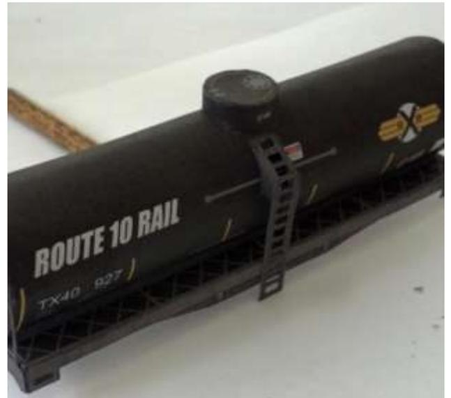
7.) Cut out the Ladder(s) – you can choose to put on 1 or 2 or none if you like. Also – you can cut out the “holes” between rungs, or just leave it solid if you wish. Glue to the Tank as shown, and also where it crosses the Deck at the bottom.
