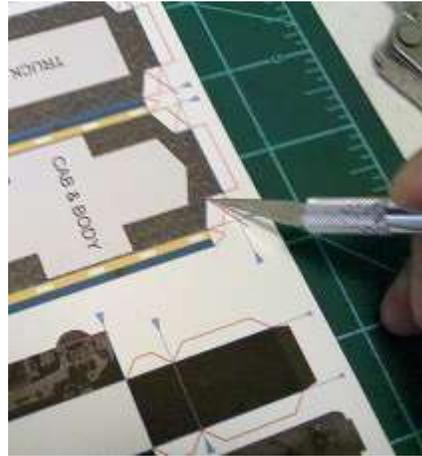
Score all Blue lines prior to cutting parts from sheet. This can be done with any blunt blade, like a dull butter knife, or other thin blade that will not cut the paper. Use a metal ruler, or metal-edged ruler to keep lines straight. Blue Guide Arrows are provided where possible, however, there are fold lines that arrows cannot be placed on, so look closely for those.
