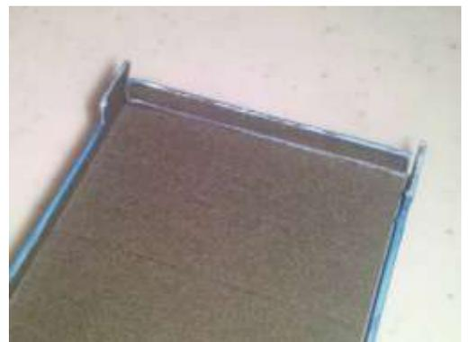
5.) Glue ends into place, then glue down the bottom backside of the end flaps to complete the “recessed” belly area.
