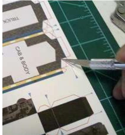
Score all Blue lines prior to cutting parts from sheet. This can be done with any blunt blade, like a dull butter knife, or other thin blade that will not cut the paper. Use a metal ruler, or metal-edged ruler to keep lines straight. Blue Guide Arrows are provided where possible, however, there are fold lines that arrows cannot be placed on, so look closely for those.
